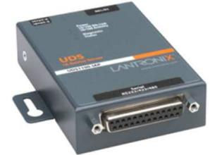
The UDS1100-IAP is a rugged and powerful tool which enables users to connect, manage and control just about any piece of industrial equipment from virtually anywhere over Ethernet or the Internet.
